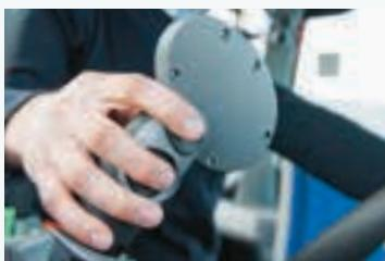
The button on the rear of the CommandGrip™ gives access to further functions.
