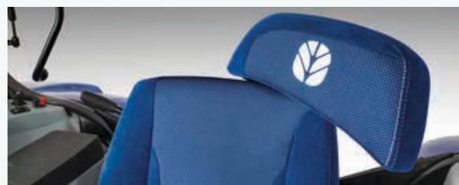
Both the Dynamic Comfort and Comfort seats benefit from the innovative swiveling backrest, designed to provide upper back support and significantly increases comfort when the seat is turned to monitor rear mounted implements.
