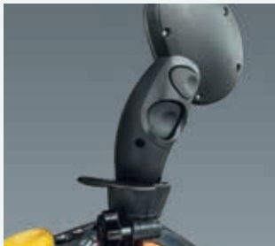
Shift button and ground speed unlock (behind).
