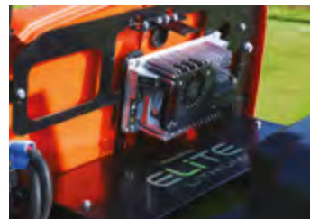
ELITE lithium battery & on-board high frequency 18 amp, 48V DC output, 85 - 265V AC 45 - 65 Hz input
