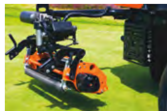
Easy access swing-out centre cutting unit
