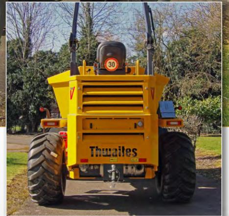
The Thwaites 9 Tonne Power Swivel, Stage V dumper is manufactured with contractors and hirers in mind – ensuring operator safety, reducing risk on site, and improving performance. The Power Swivel skip enables a 90° rotation left and right, allowing the machine easier access to tip loads in restricted areas, giving the operator greater control and reducing risk on site.
