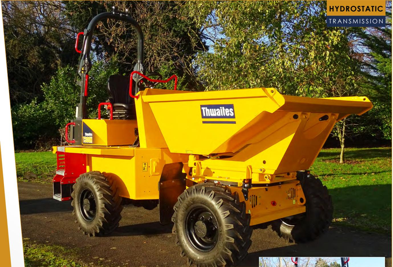
The Thwaites T300H Hi Swivel, Stage V dumper is manufactured with contractors and hirers in mind – ensuring operator safety, reducing risk on site and improving performance. Powered by a 33.3 kW Yanmar engine, delivering 142 Nm max torque for optimum traction and control, this machine is driven by a Hydrostatic transmission, making it simple and straightforward to operate.
