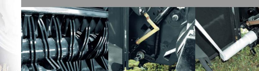
Heavy duty floor roller provides gentle but firm rotation while supporting the weight of the bale.
