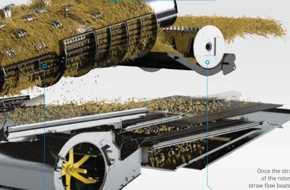
Once the straw has reached the end of the rotors, the 400mm diameter straw flow beater moves straw onto the positive straw discharge belt. This belt directs the straw rearwards, for efficient flow through to the rear of the combine.
