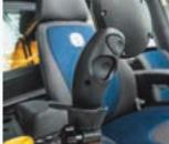
Shift button and ground speed unlock (behind).
